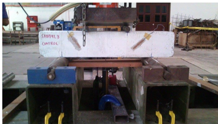
Figure 3.16: Actual arrangement of beam
