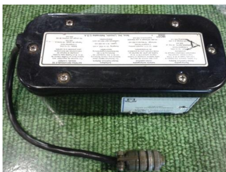
Figure 3.6: Battery of Flow-meter C4250
