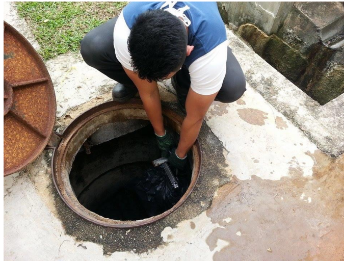
Lab assistant hangs the Flow-meter in a manhole
