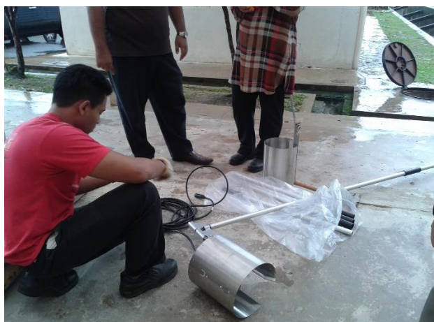
Installation of Flow Meter Sensor in mounting ring by lab assistant
