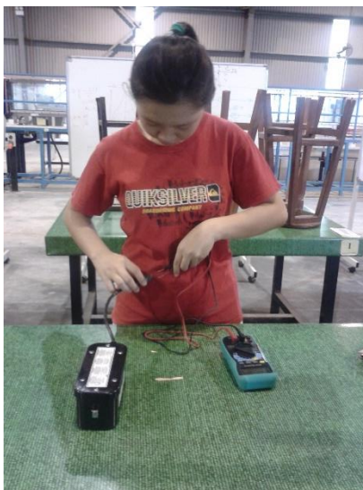
Using multimeter to check the battery voltage
