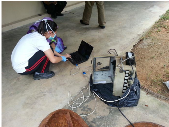
Set up the Flow-meter by using laptop
