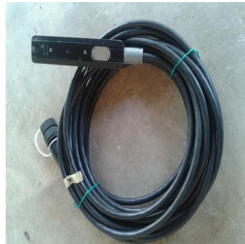
Figure 3.11: Isco Flow-meter Sensor
