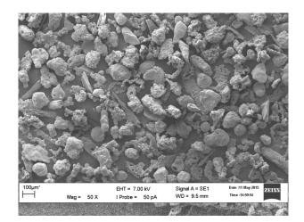
Figure 2.1: Scanning Electron Microscopy (SEM) of POFA
