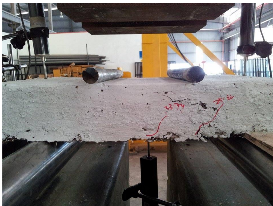
(b): Failure mode for sample 2
