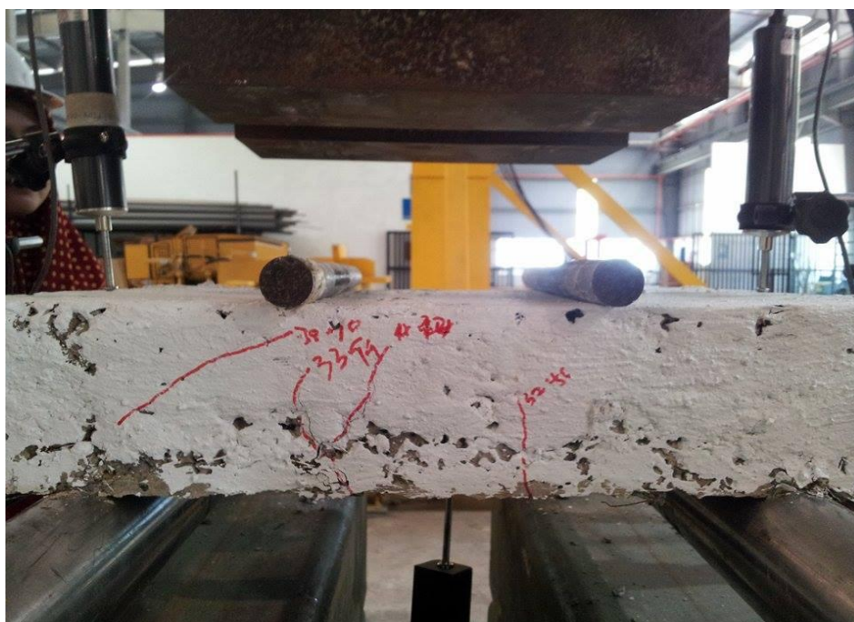
(b): Failure mode for sample 2
