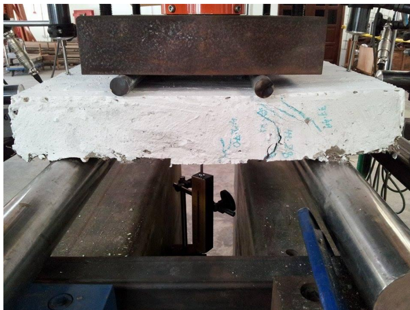
(c): Failure mode for sample 3
