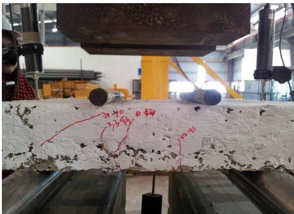
(b): Failure mode for sample 2
