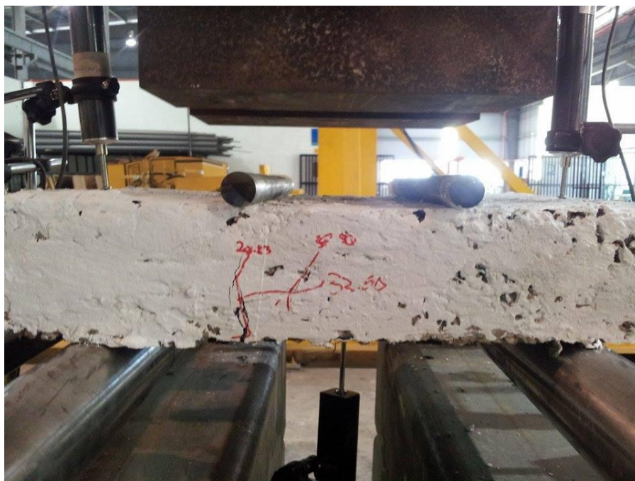
(a): Failure mode for sample 1
