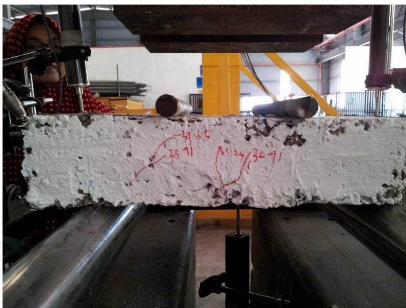
(b): Failure mode for sample 2
