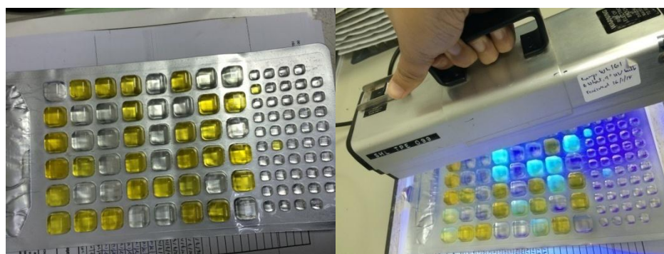
Figure 3.4: Most Probable Number (MPN) method
