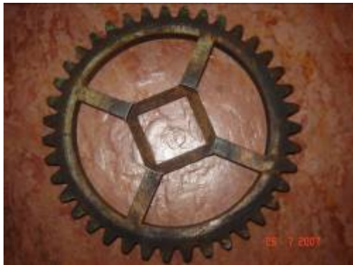
Fig. 3: The end shape of the work piece after wire-EDM cutting process
