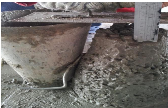
Figure 3.20: Slump test for concrete
