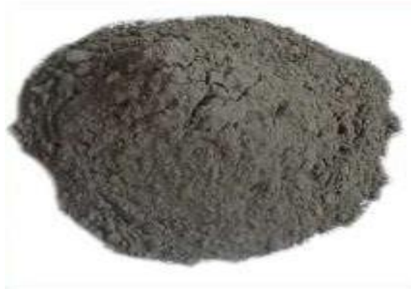
Figure 3.2: Ordinary Portland Cement is grey in colour
