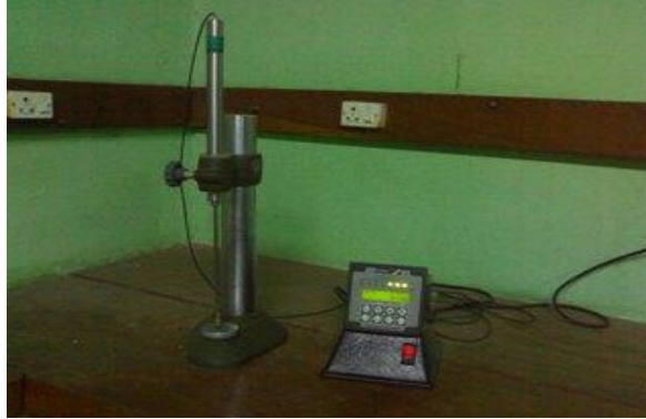
Figure 3.23: LVDT is used to measure the deflection of specimen
