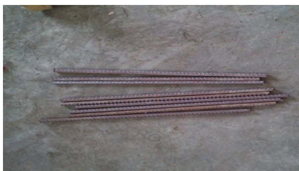
Figure 3.7: Steel bars are used in this research to reinforce the concrete slab
