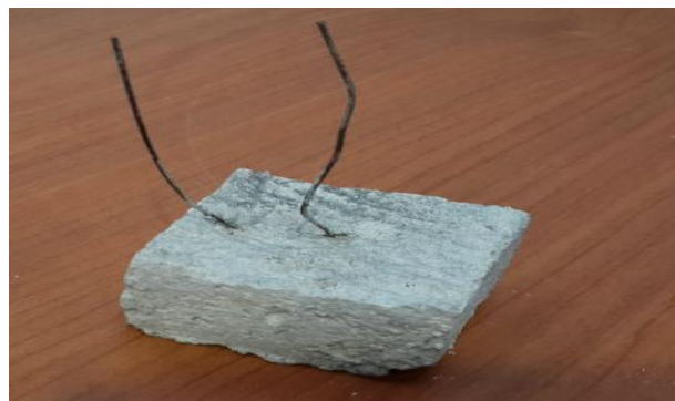
Figure 3.14: The size of concrete cover used in this research is 25 mm
