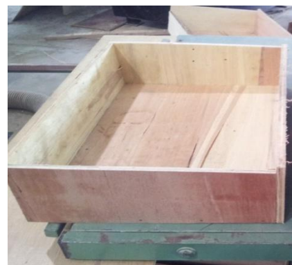
Figure 3.12: Prepared slab formwork
