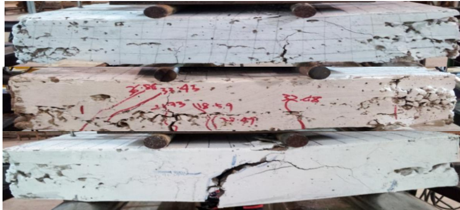
Figure 4.11(c): Failure mode of slabs B3 after testing
