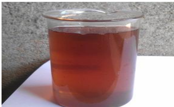
Figure 3.8: Superplasticizer is measured to a required amount in a beaker
