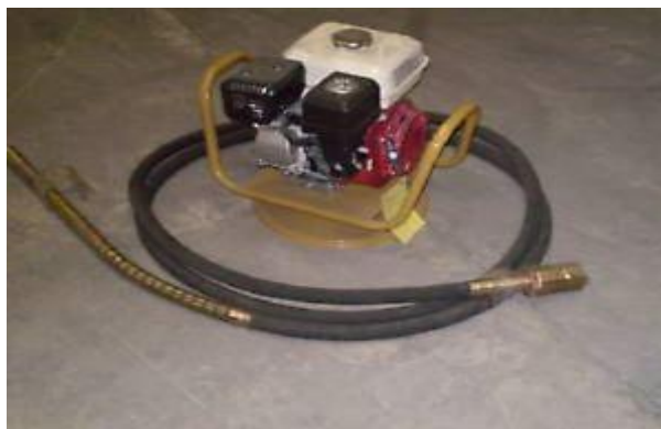
Figure 3.16: Poker Vibrator which is used for compaction of concrete
