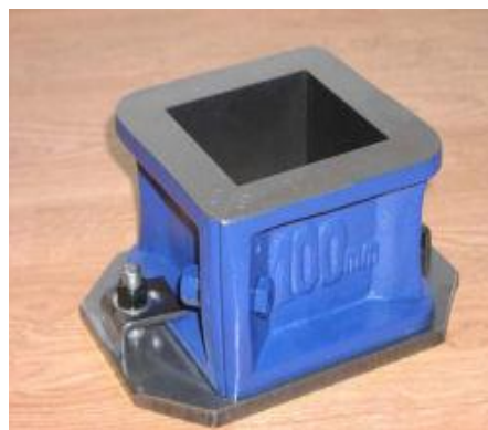
Figure 3.11: Prepared cube mould
