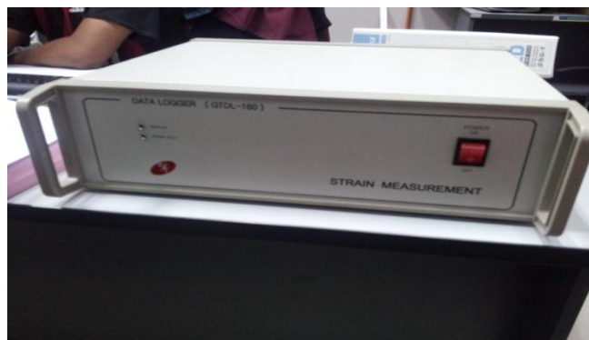
Figure 3.25: Data Logger is used to record the measurements of specimen
