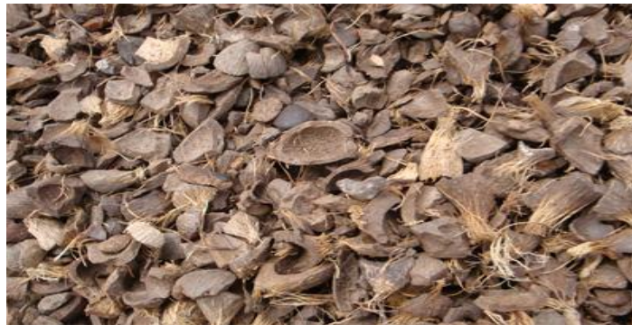
Figure 3.5: Crushed oil palm shell
