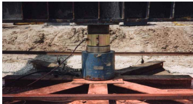
Figure 3.24: Hydraulic Jack Load is used to transfer load to the specimen
