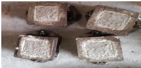
Figure 3.17: Hardened cube before dismantling from mould
