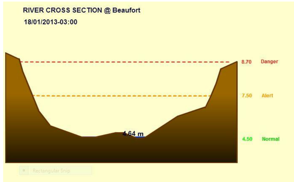
FIGURE 3 SHOWS THE CROSS SECTION OF THE RIVER AT THE BEAUFORT WATER LEVEL STATION. (PICTURE IS COURTESY OF INFOBANJIR.GOV)
