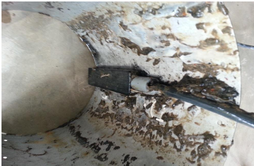
Figure 4.20: Obstacle is blocking the sensor to detect the flow rate
