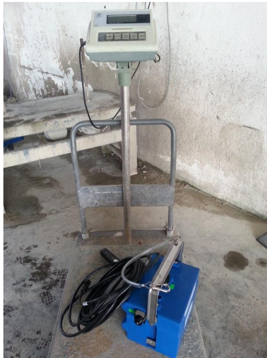
Figure 3.2: Weighting flowmeter (including batteries and sensor)
