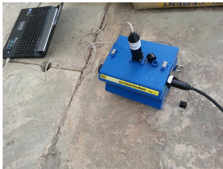
Figure 3.8: Flowmeter cable adaptor is connected to the computer
