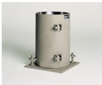
Figure 3.6: Mould for cylinder
