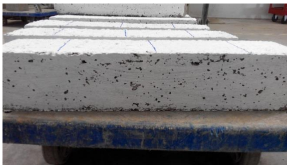
(a) Prism specimen ready to assemble in flexural machine
