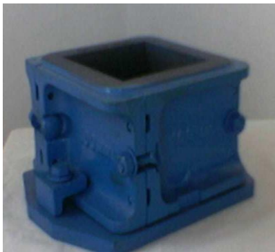
Figure 3.5: Mould for cube
