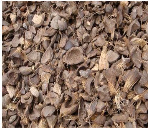
Figure 2.1: Sample of OPS aggregate
