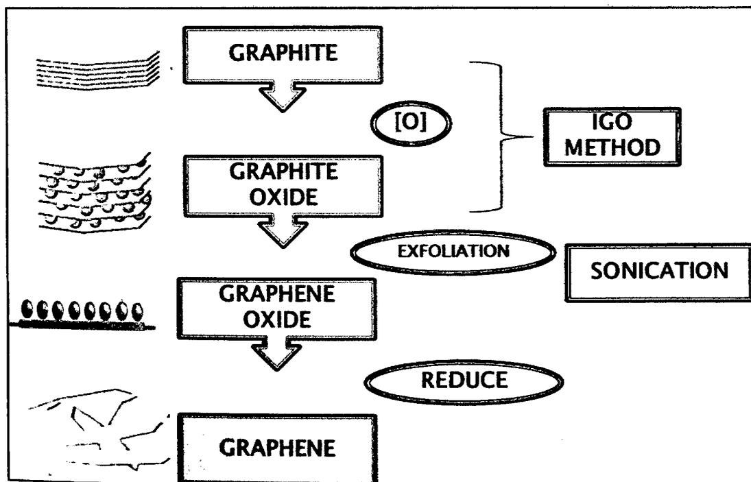
Figure 3.2: Process Flow Diagrams for the Synthesis of Graphene from Graphite
