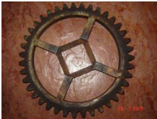
Fig. 3 The end shape after wire-EDM cutting process
