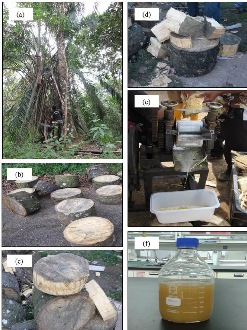
Figure 3.1: OPT sap preparation. (a) Oil palm tree was cut down (b) The trunk was cut into pieces (c) The trunk bark was removed (d) The middle part of the trunk was cut into smaller pieces (e) The trunk pieces was squeezed through the sugarcane machine (f) The sap obtained was filtered and stored.
