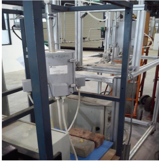
Figure 3-7: Gas Catalytic Reactor with Vertical Tube reactor
