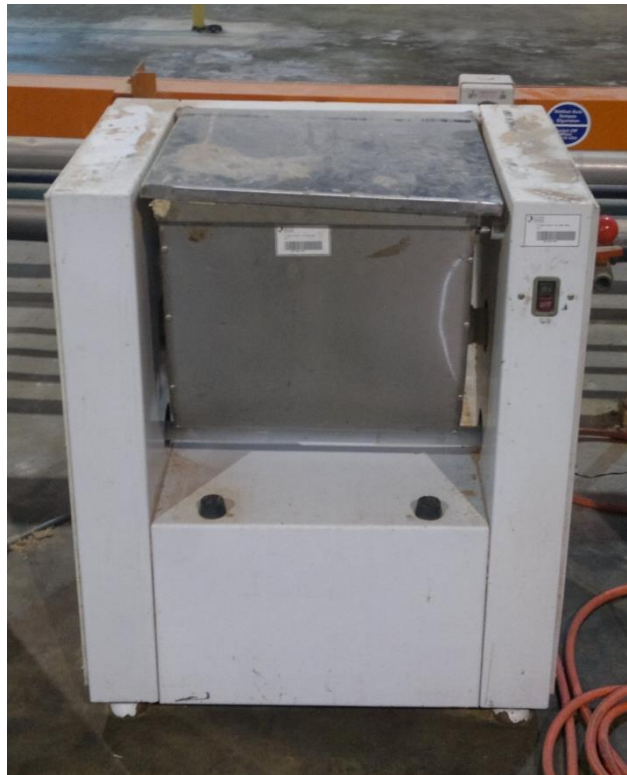
Figure 2.3.3.1-1: Picture of the glue blender or the rotatory drum that is used in the preparation of wood fibres for MDF (personal)
