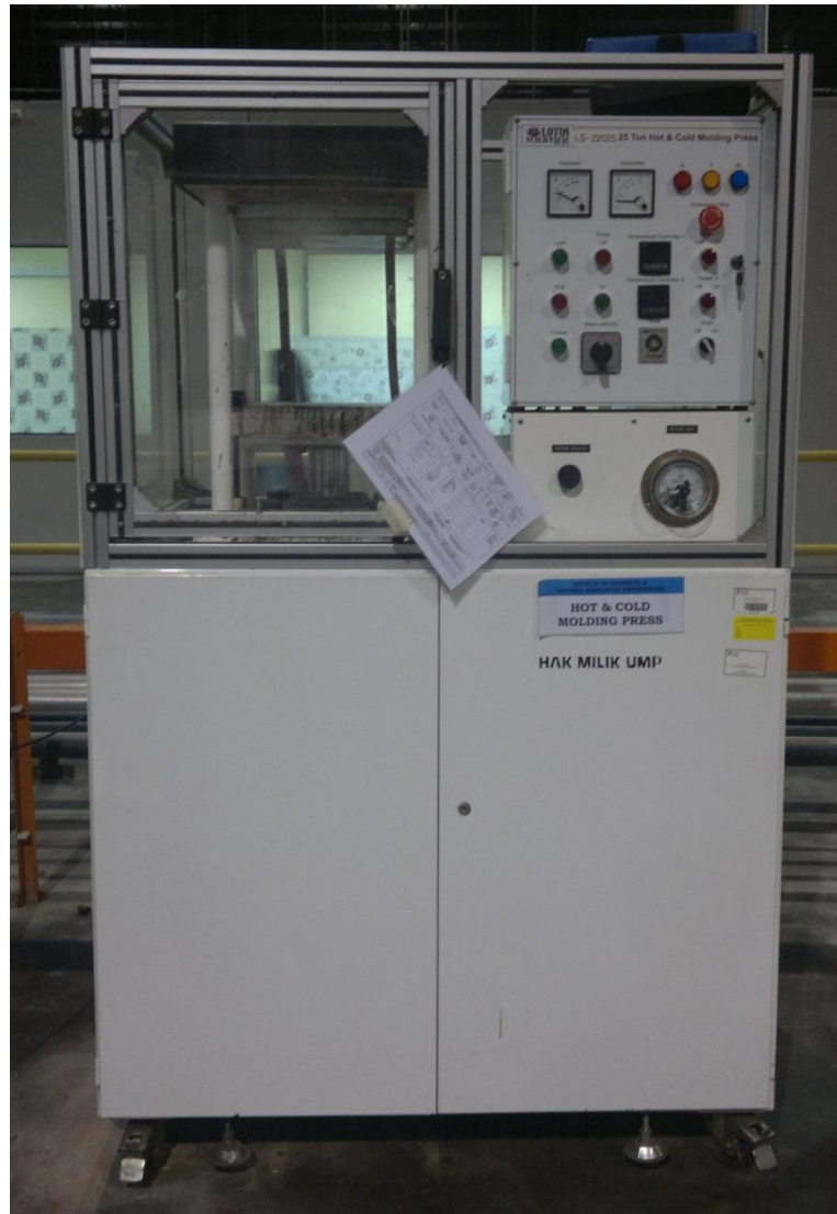
Figure 2.3.3.1-3: The hot and cold press machine which is responsible for the fabrication of MDF (personal)
