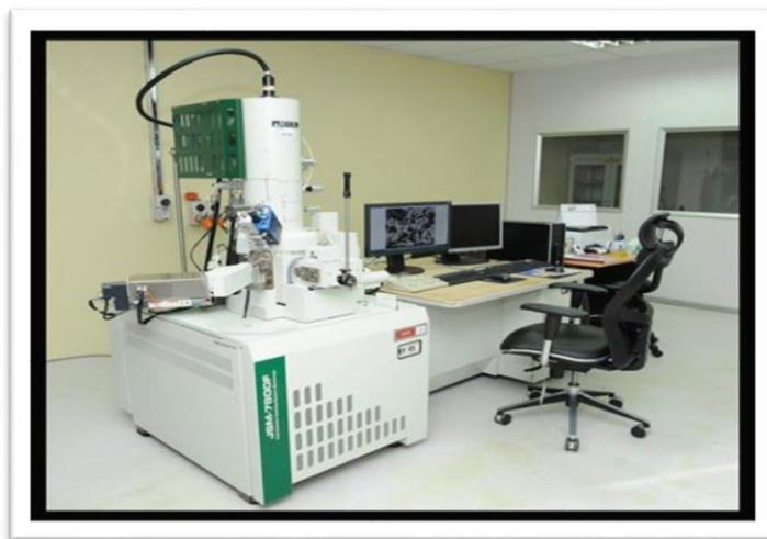
Figure 3-2: Scanning Electron Microscopy (SEM).
