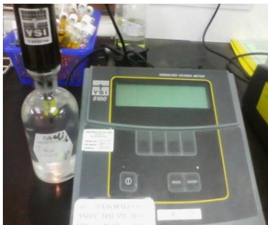
Figure 3-8: Dissolved oxygen meter.
