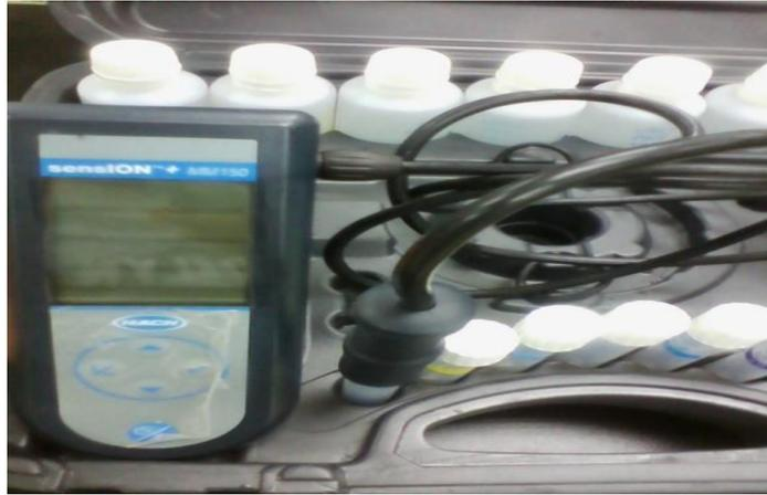
Figure 3-6: pH, conductivity and TDS meter.
