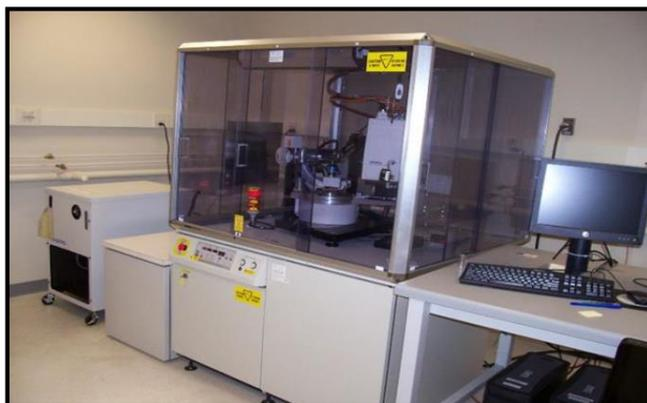
Figure 3-4: X-Ray Diffraction (XRD).
