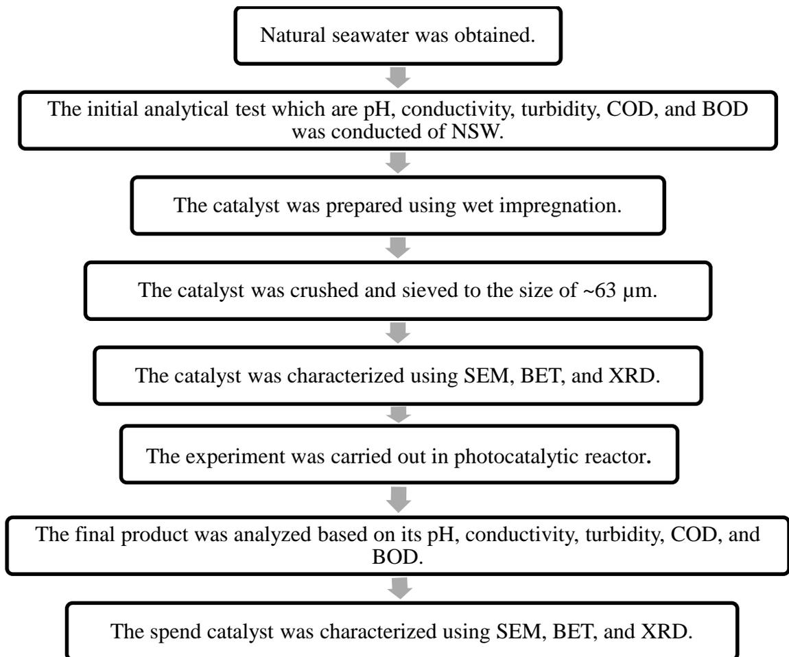
Figure 3-1: Flow diagram of experimental procedure.
