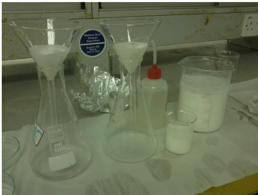
Figure A2: Filtration and washing of ZnO solution
