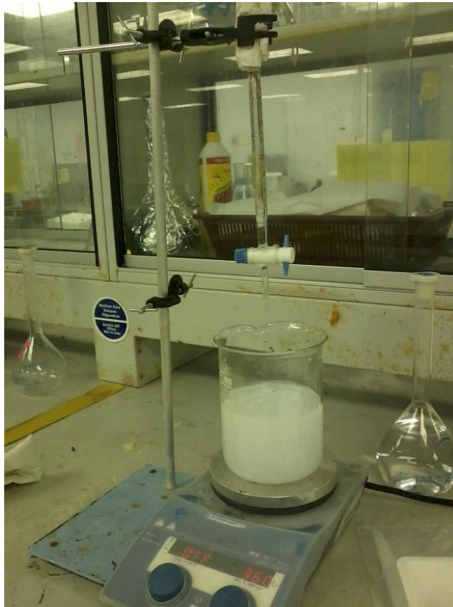
Figure A1: Mixing process to produce ZnO nanoparticle
