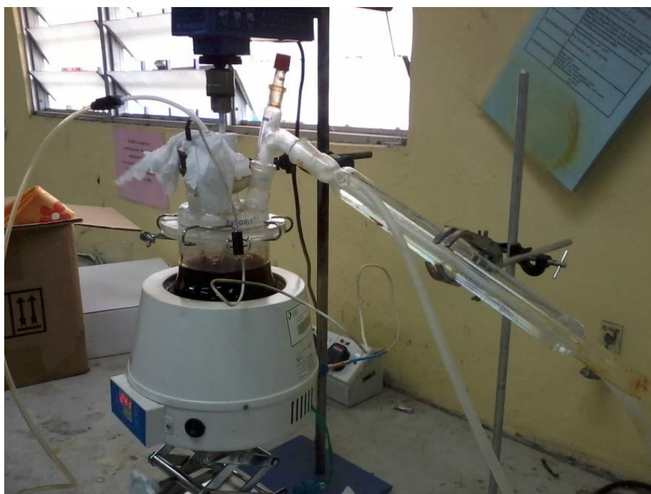
Figure A4: Two stages alcoholysis-polysterification process
