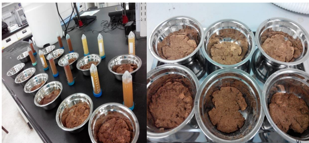
c) OPF sample after washing. The pulp will be dry in oven for 24 hour
