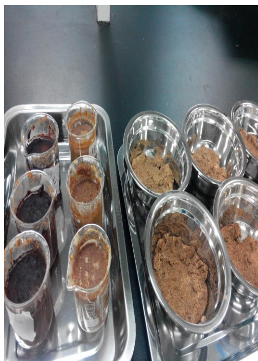
Figure 3-2: Left : OPF sample that has been pre-soaked in mixture of lime and NaOH concentration.
