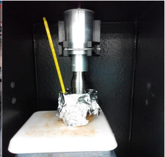
f) OPF sample being heated using method ultrasonication by ultrasonic probe for certain time
