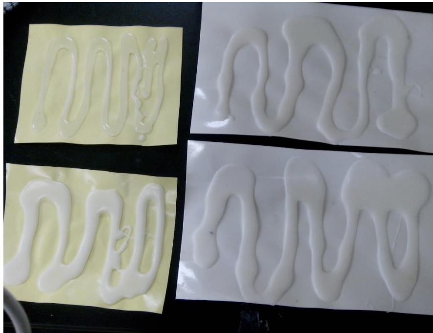
Appendix C.3: EVA hot melt adhesive on silicon paper at ambient temperature
