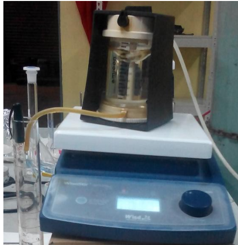
Figure 3-4 Dead end test set-up
