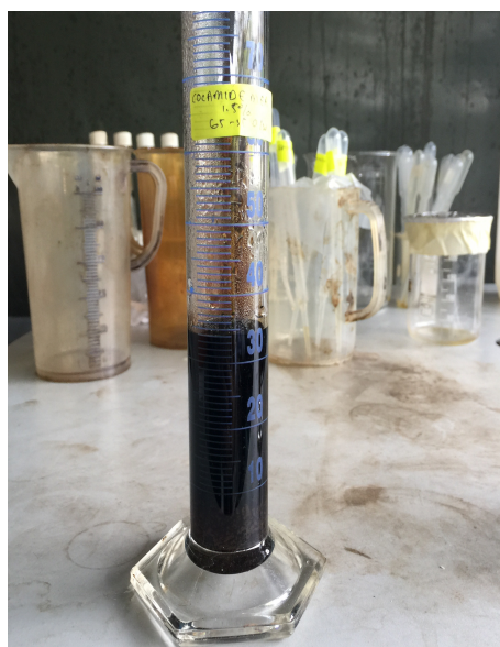
Figure 4.6.31: Ratio of 65/35 Emulsion with Demulsifier MEA 1.5
