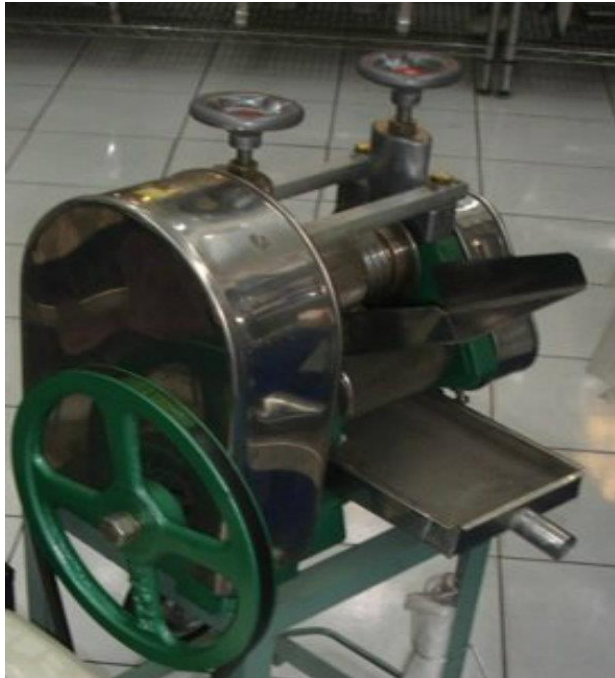
Sugarcane machine was used to press the banana stem.
