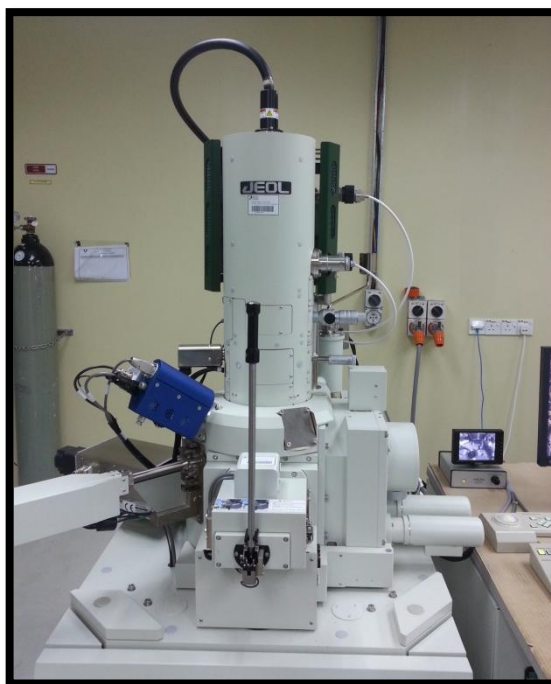
Figure 3-12 : Scanning electron microscopy device that was used to observed catalysts
