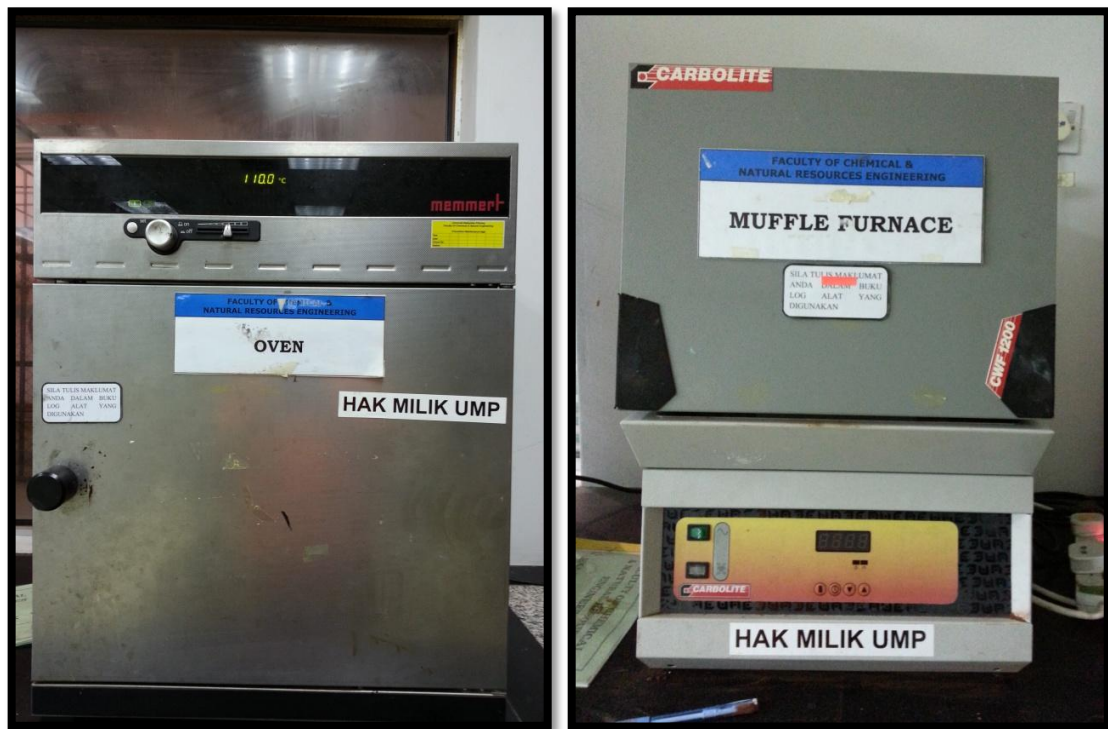
Figure 3-7 : Oven (left) and muffle furnace (right)
