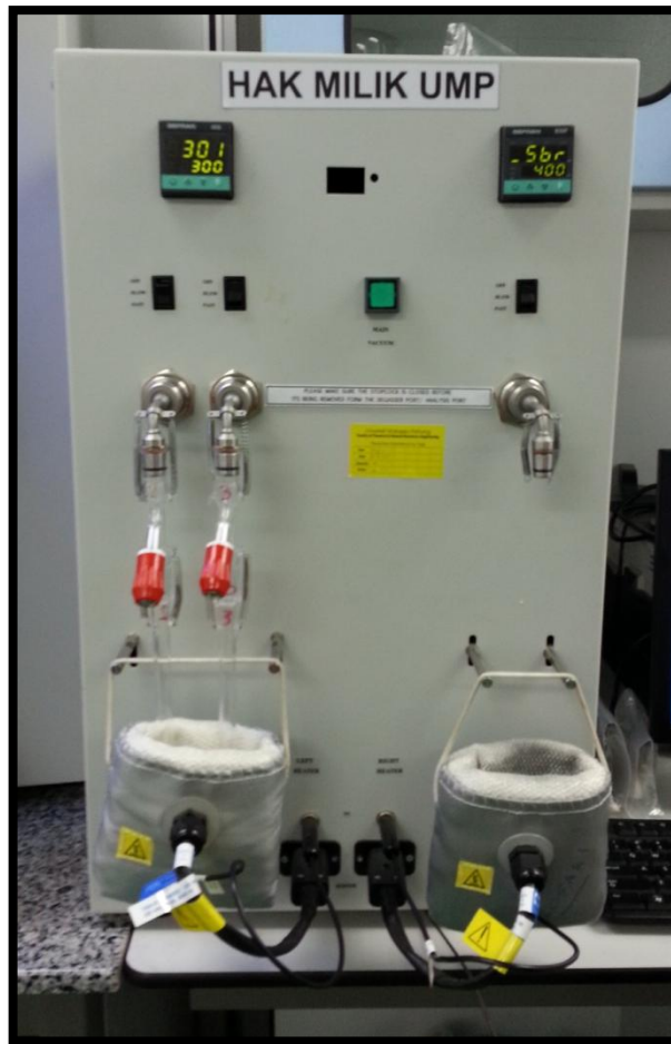
Figure 3-9 : BET device used for characterization
