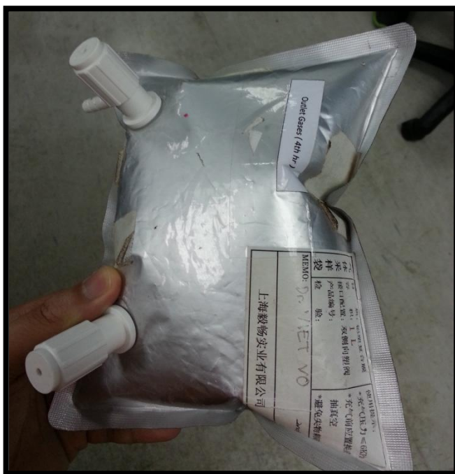
Figure 3-17 : Example of gas bag that was used to transfer product gas to be analyzed in Gas chromatography.
