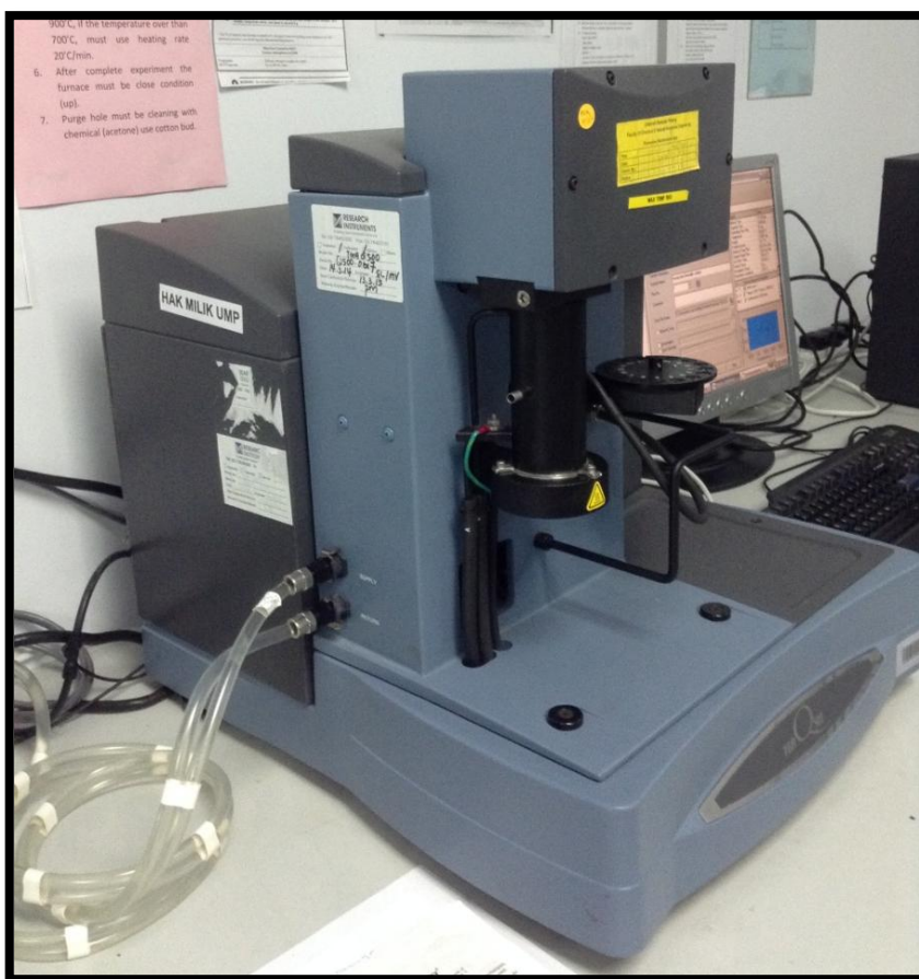
Figure 3-13 : TGA (Research instrument, model: TGA Q500)
