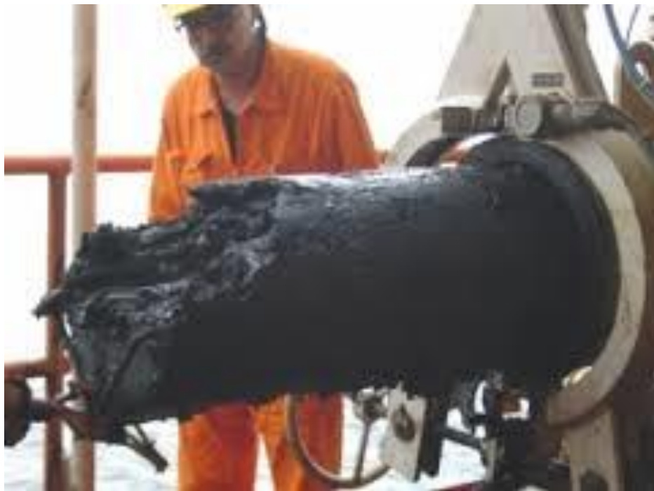
Figure 2-1: Wax deposition in pipeline
