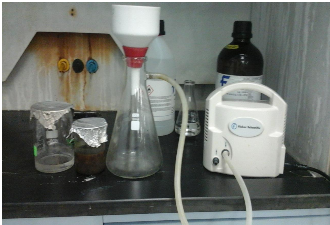
Figure 3-9: Extraction of Waxy Crystal from crude oil
