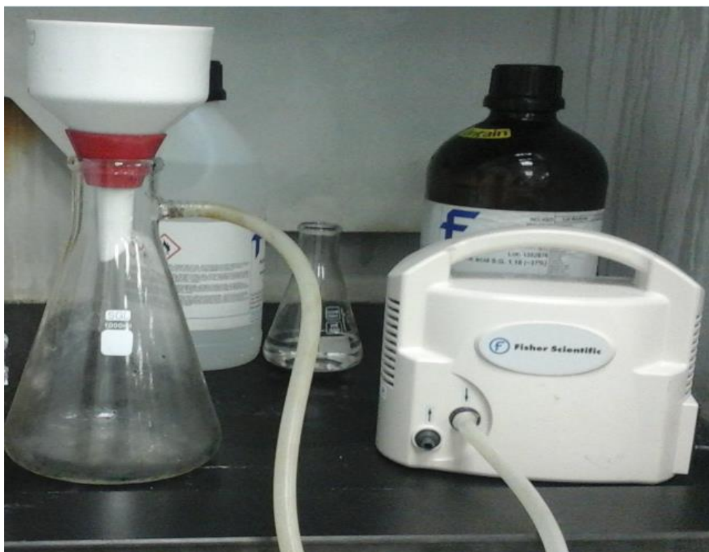
Figure 3-10: Asphaltene Precipitation Process
