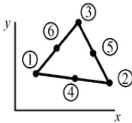
Figure 1: Six-node quadratic triangular elements
