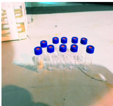
Figure B-1.5: Sample from upper and lower phase were mixed with n-heptane in 1 ml vial and GC analysis was conducted
