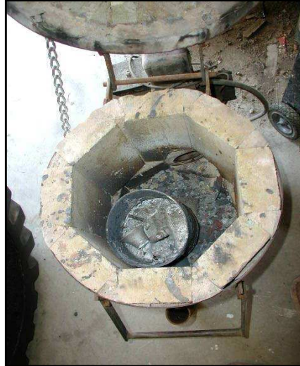
Figure 2.5: Combustion chamber of furnace
