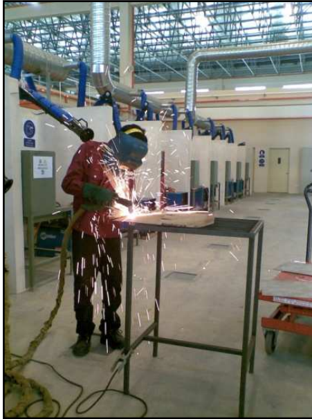
Figure 3.15: Using plasma cutting machine
