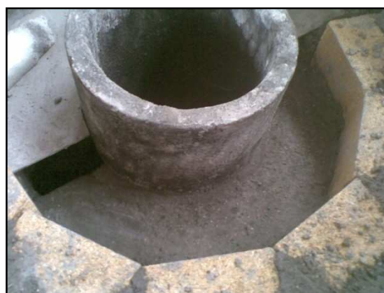
Figure 3.20: Graphite crucible support by buffers
