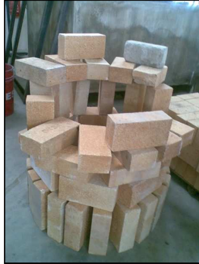
Figure 3.13: A few of firebricks
