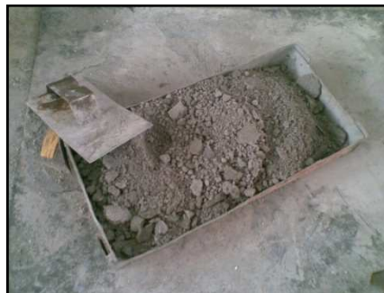
Figure 3.14: Castable before mix up with water
