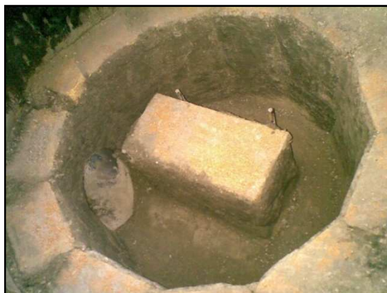
Figure 3.19: Firebricks under the crucible
