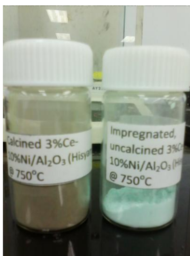
Figure 3-5: Impregnated, calcined and uncalcined 3%Ce-10%Ni/Al 2 O 3
