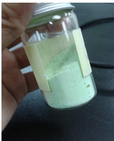
Figure 3-4: Impregnated, uncalcined 3%Ce-10%Ni/Al 2 O 3
