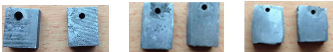
Figure 3: Comparison of surface condition of different percentage cold working aluminium anodes.
