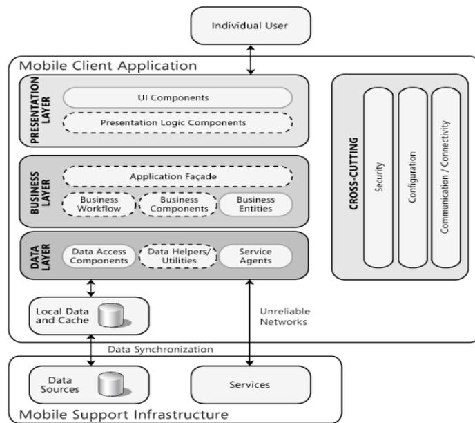
**Figure 2.10:** Common mobile application architecture
