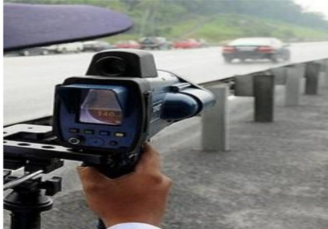
**Figure 2.3:** Example of speed trap camera
