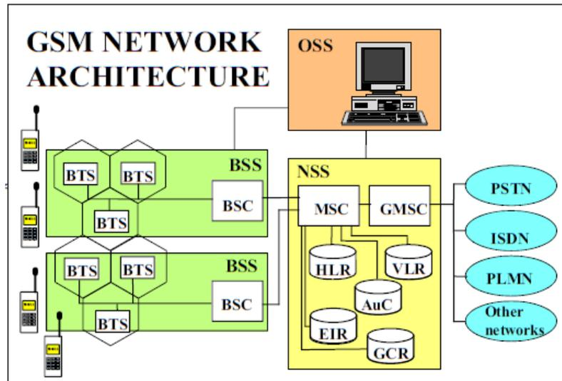
**Figure 2.5:** GSM network architecture
