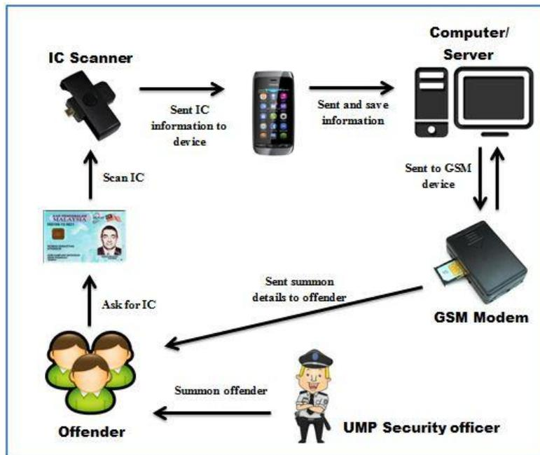
**Figure 3.1:** Complete context diagram of E-Saman system
