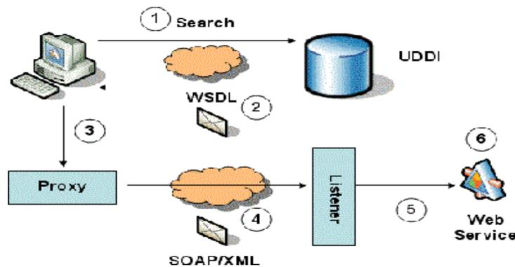
**Figure 2.7:** The process flow of a Web Service
