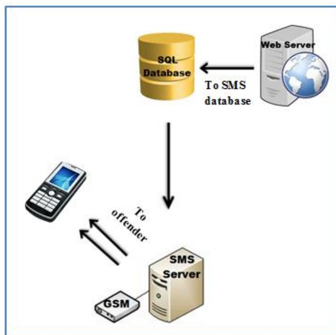
**Figure 3.6:** Logical diagram of GSM system
