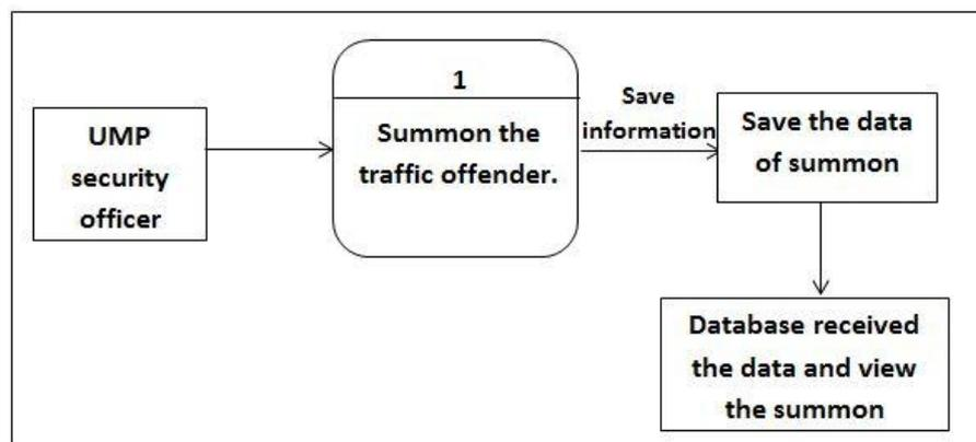
**Figure 3.3:** DFD level 0 for UMP security guard office summon the offender
