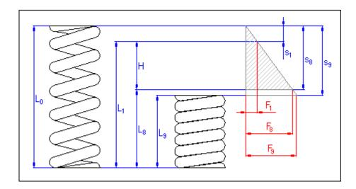
Figure 2.10 The States of the Spring According to Index of Basic State of Springs [35]
