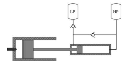
Figure 2.6 A Single Piston Hydraulic Free Piston Engine [28]
