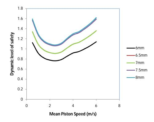
Figure 4.4 Dynamic Level of Safety versus Mean Piston Speed
