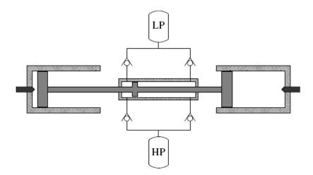
Figure 2.7 Dual Pistons Hydraulic Engine [28]
