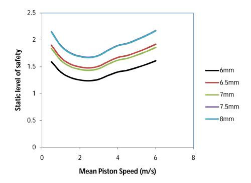
Figure 4.5 Static Level of Safety versus Mean Piston Speed
