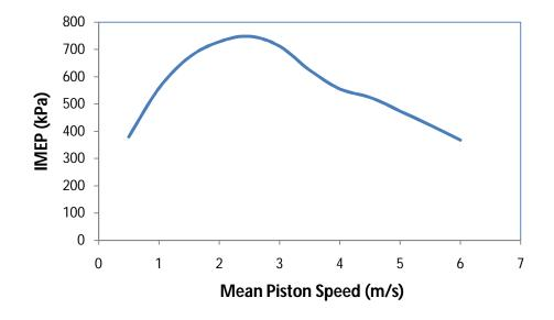
Figure 4.1 IMEP versus Mean Piston Speed of Linear Engine
