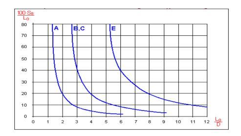
Figure 2.14 Curves of Permitted Deformation According to the Type of Seating of the Spring [35]
