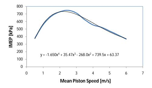
Figure 4.2 Polynomial Interpolation of IMEP versus Mean Piston Speed
