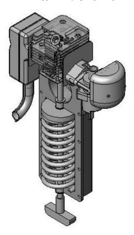
Figure 4.8 Isometric View of Linear Engine
