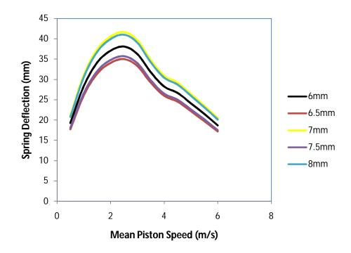
Figure 4.3 Spring Deflection versus Mean Piston Speed
