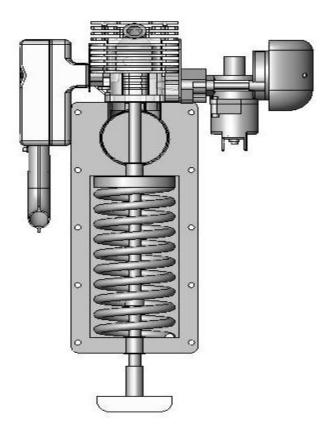
Figure 4.12 Spring at Preloaded Condition
