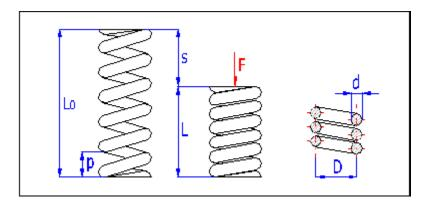
Figure 2.11 Helical Cylindrical Compression Spring [35]
