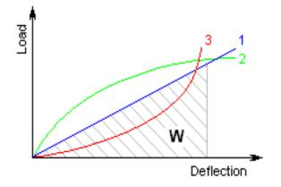
Figure 2.9 Spring Characteristic Curve [35]
