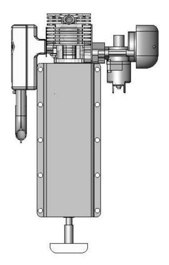
Figure 4.9 Front View of Full Assembly Linear Engine
