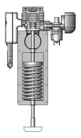
Figure 4.13 Spring at Fully Loaded Condition
