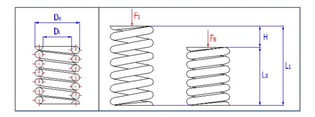
Figure 3.6 Input Parameters Applied to the Spring [35]
