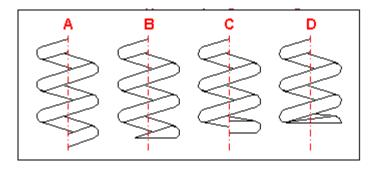
Figure 2.12 Common Types of Spring End Designs [35]
