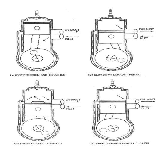
Figure 2.4: Working Principle of Two-Stroke Engine [21]
