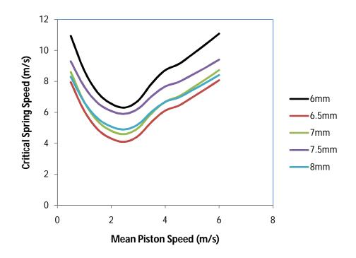
Figure 4.6 Critical Spring Speed versus Mean Piston Speed
