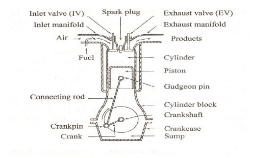
Figure 2.2 Cross Section of a Single Cylinder Spark-Ignition Engine [7]
