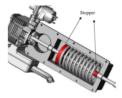
Figure 4.11 Location of Stopper in Linear engine
