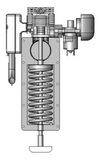
Figure 3.8 Designed Linear Engine
