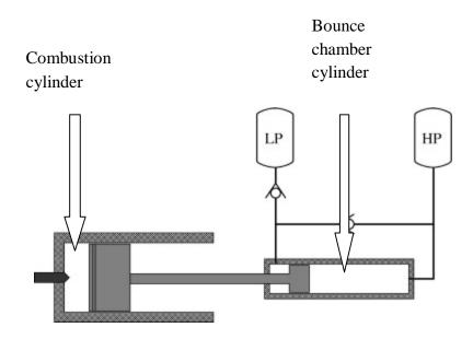
Figure 2.5 Basic Concept of Free Piston Engine [28]
