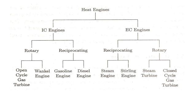
Figure 2.1 Detailed Classifications of Heat Engines [7]
