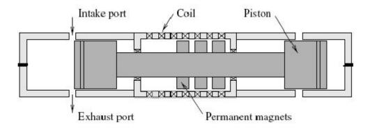
Figure 2.8 Illustration of the Free Piston Engine Generator [28]
