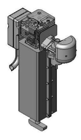
Figure 4.10 Isometric View of Full Assembly Linear Engine
