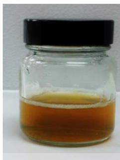
**Figure 3.3:** HEC with 0.8% silver nanoparticles blended solution
