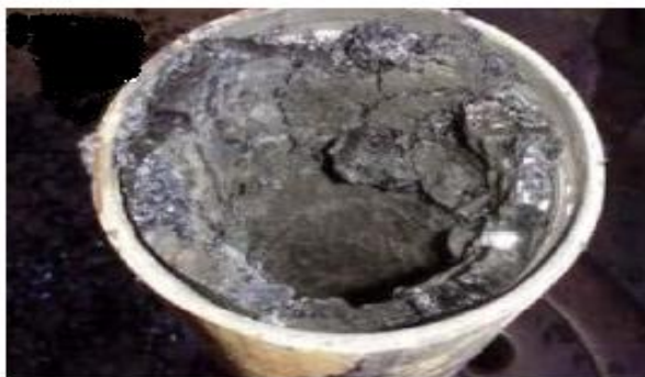
Figure 1.2: Asphaltenes deposited in the pipeline
