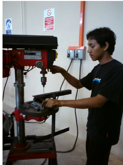
Figure 3.17: Using press drill
