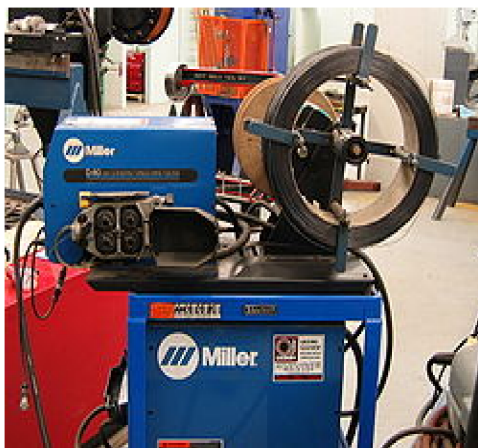
Figure 2.3: Metal Inert Gas (MIG) Welding
