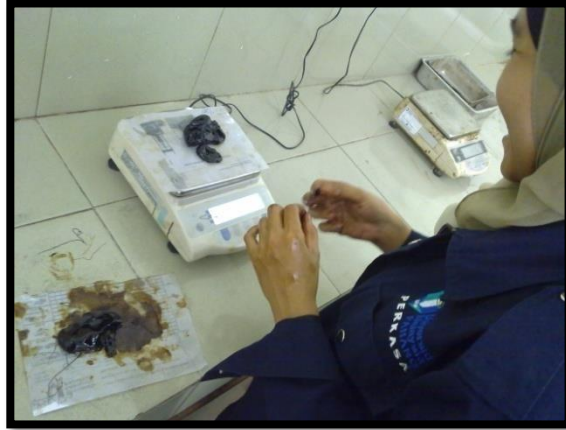
Figure 3.4: Asphalt is weighted.
