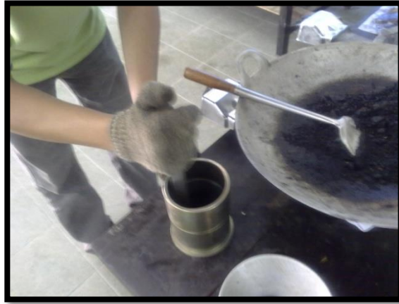
Figure 3.5: Sample was compacted into the mould
