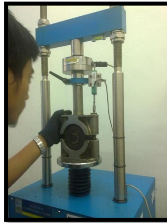
Figure 3.7: The sample was placed in the testing head.
