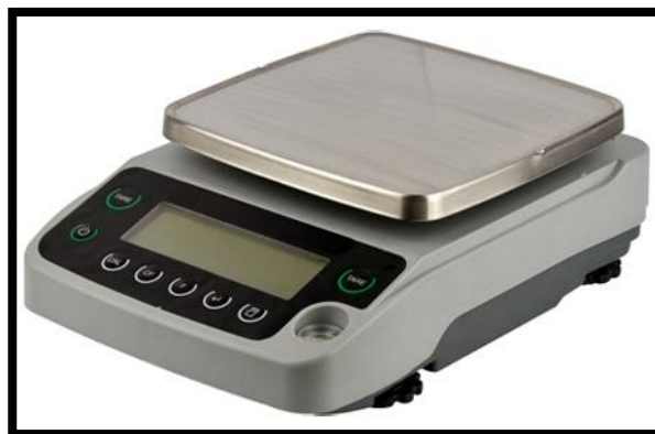
Figure 3.3: Analytical balance for weighing the aggregates and asphalt.
