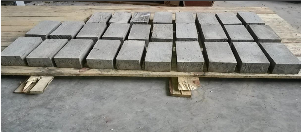
Figure 3.9: Bricks that has been removed from fromwork
