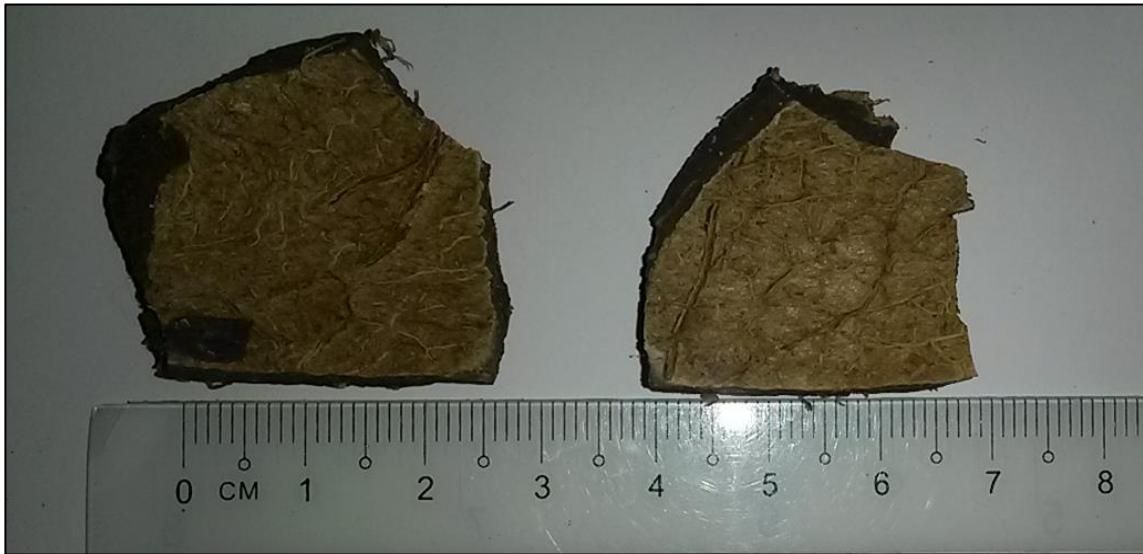
Figure 2.3.5: Size of Crushed Coconut Shells (25 mm to 30 mm)
