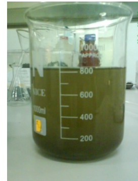
Figure A-14 : 1g of sample dissolve in 1L of distilled water ready to test.
