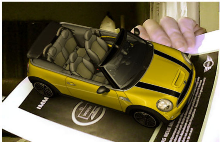
Marker transformed into 'augmented reality' when held in view of a webcam. Output as displayed on a computer screen.
