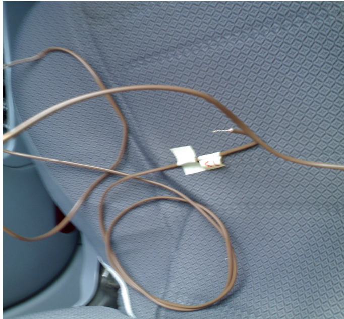
Figure 3.6: Thermocouple attach at front seat (position 3)
