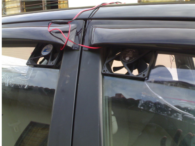
Figure 3.13: Fan is attached to the car windows
