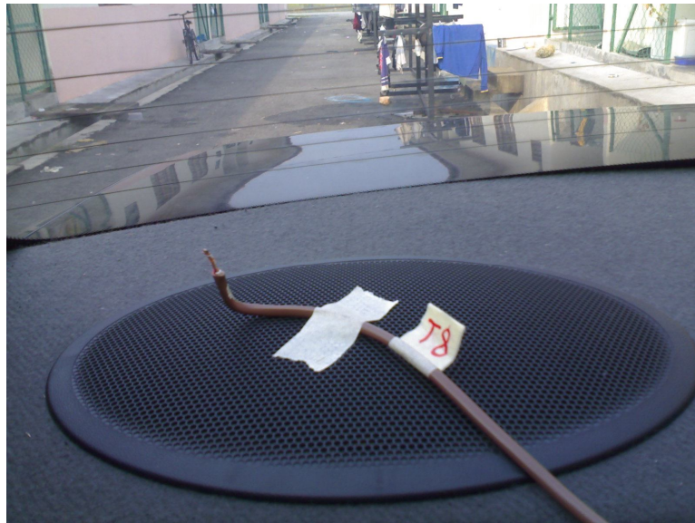
Figure 3.11: Thermocouple attach at rear panel (position 8)
