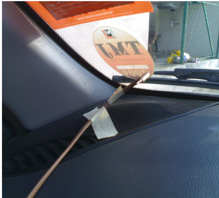
Figure 3.4: Thermocouple attach at front dashboard (position 1)
