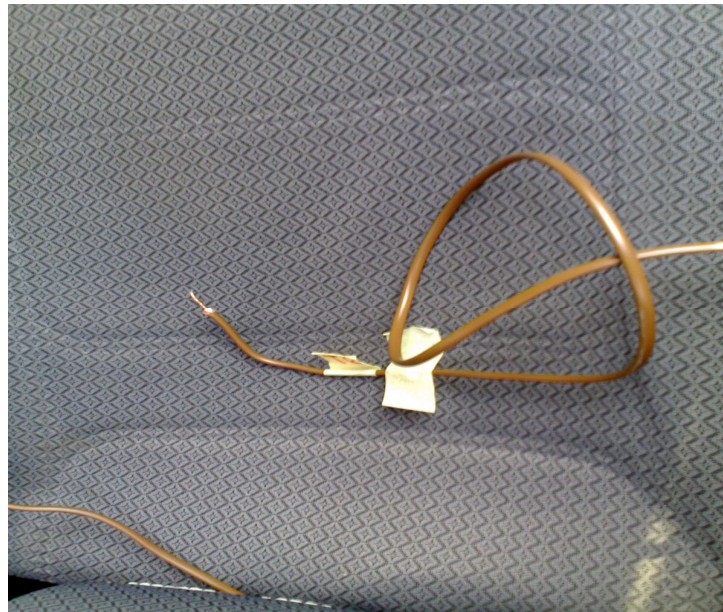
Figure 3.9: Thermocouple attach at rear seat (position 6)
