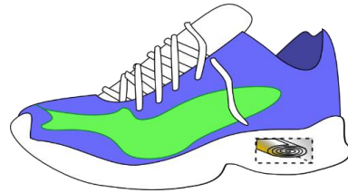
Figure 1.1: Typical implementation of microstructure device using the piezoelectric inside the shoe as the power generator
