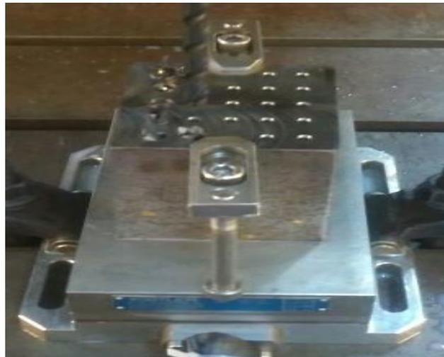
**Figure 3.3(a):** The workpiece on the dynamometer during the drilling process.
