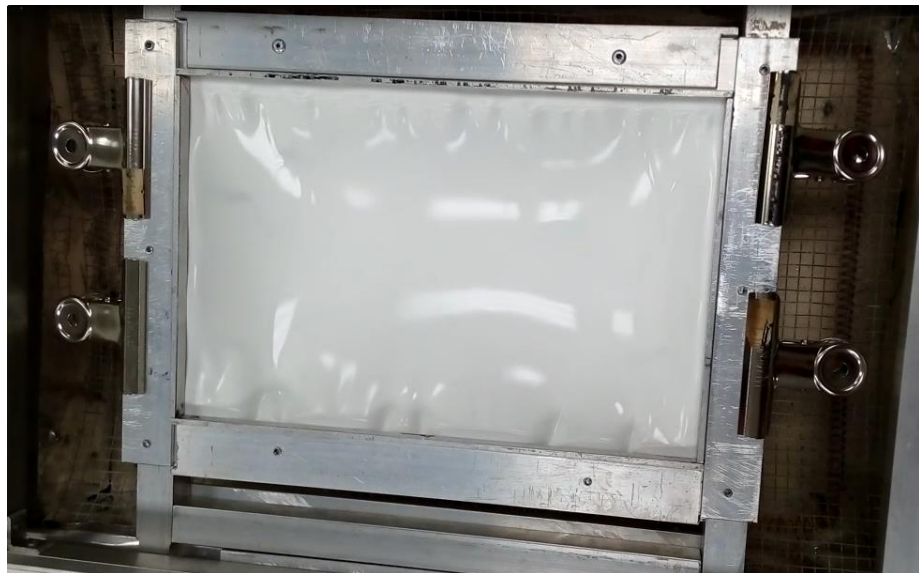
Figure 4.5: The plastic sheet at sag point
