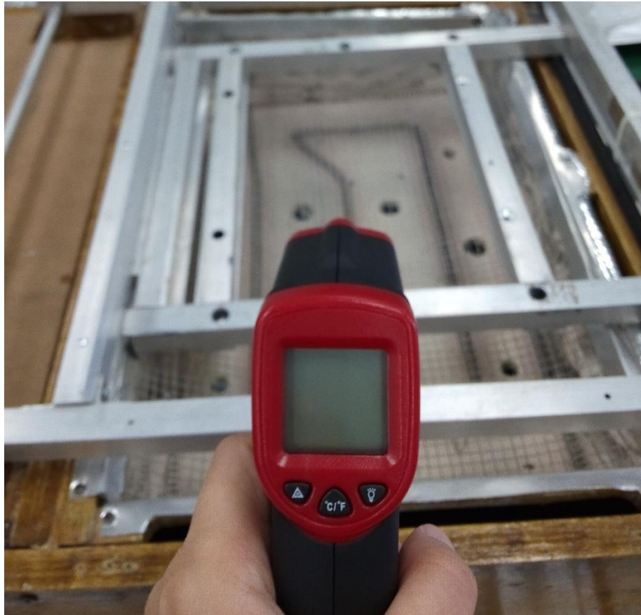
Figure 3.11: the temperature sensor used to measure temperature
