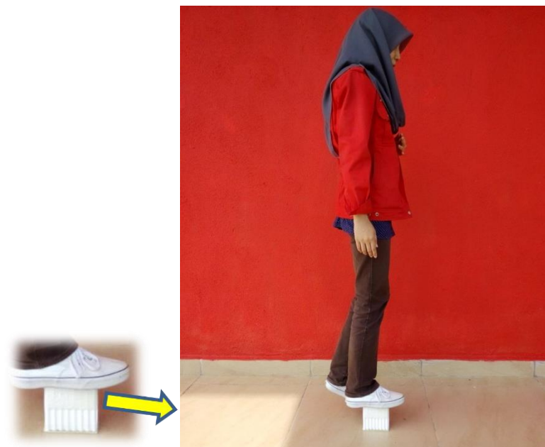
Figure 4.15: Static compression test by applying load (50kg)
