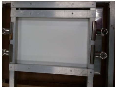
Figure 3.10: PP sheet is clamped on the clamber
