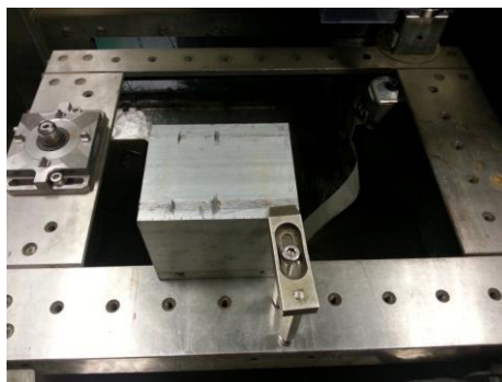
Figure 3.5: The aluminium block is clamp and ready to be machine
