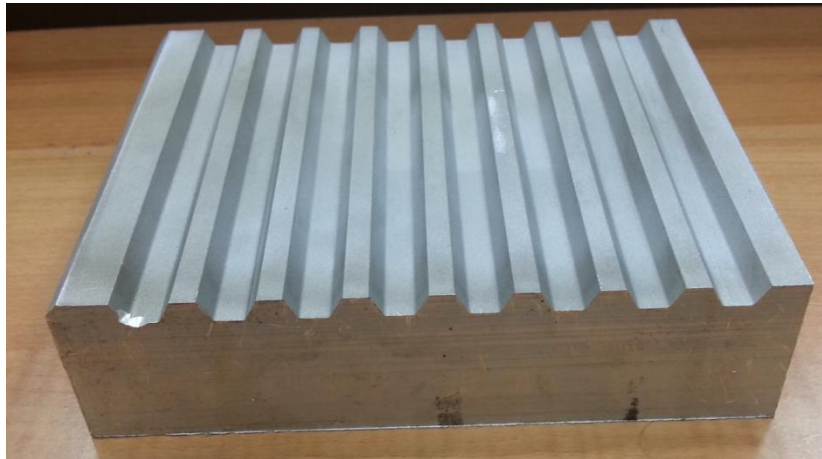
Figure 4.9: Positive honeycomb base structure mould
