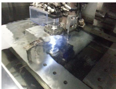
Figure 3.6: Wire-cut EDM process
