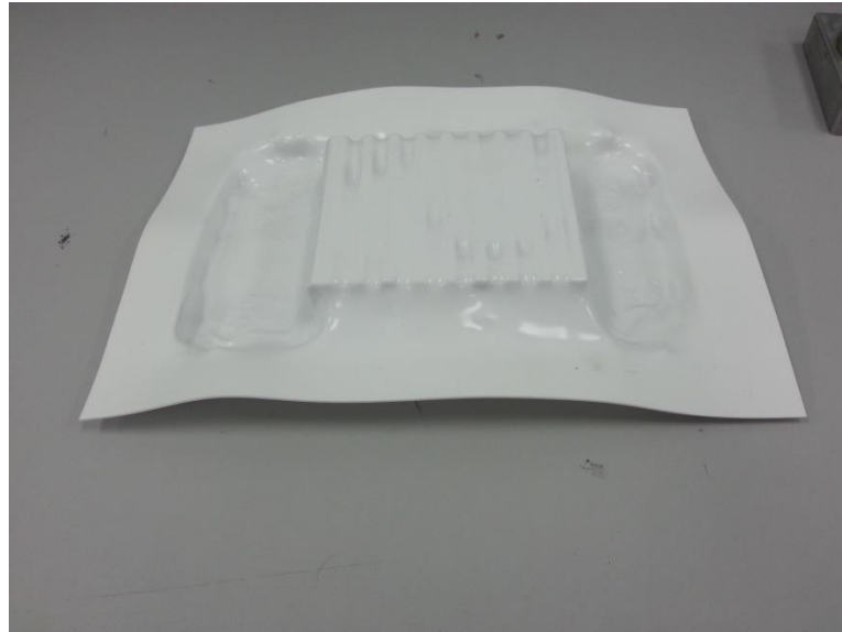
Figure 4.10: Thermoform product produced by Set up A
