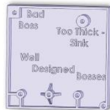
Figure 2.4: Thin bosses and draft angle
