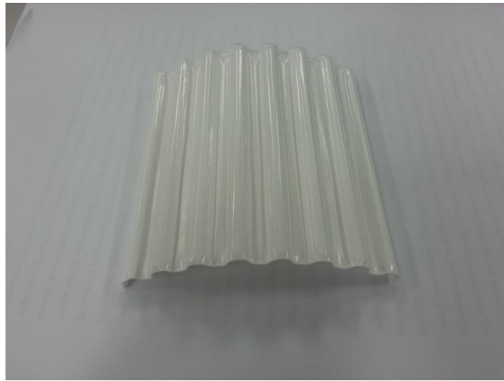
Figure 4.12: A single layer of thermoform honeycomb base structure
