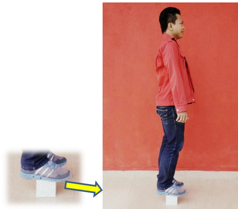
Figure 4.16: Static compression test by applying load (80kg)
