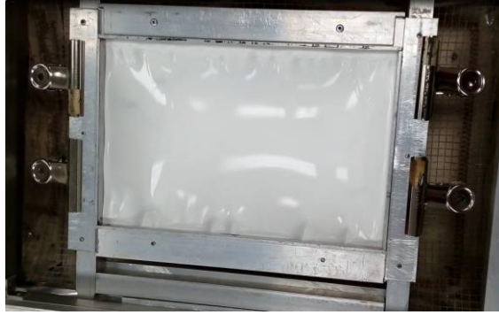
Figure 3.12: The PP sheet saggy and ready to forming process
