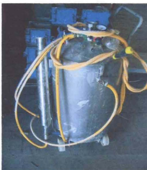
Figure 3.8 : Equipment for producing pressured foam
