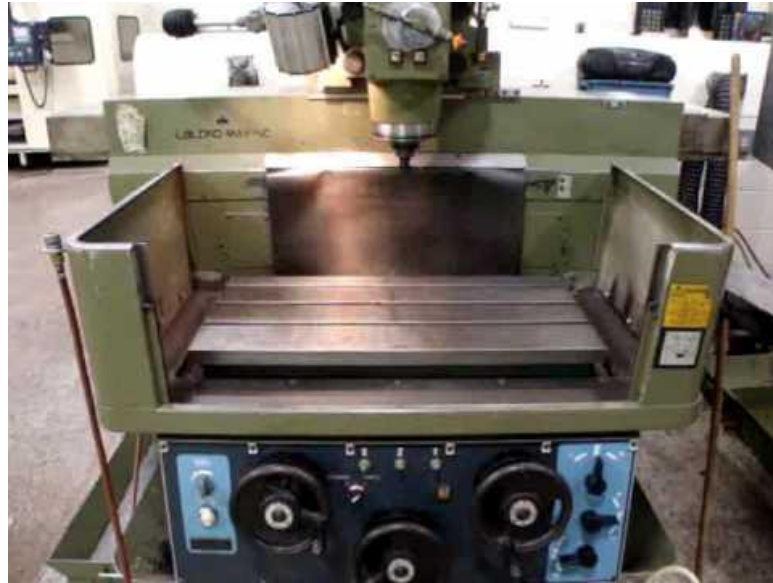
Figure 3.3: 3-axis Makino KE55 CNC milling machine
