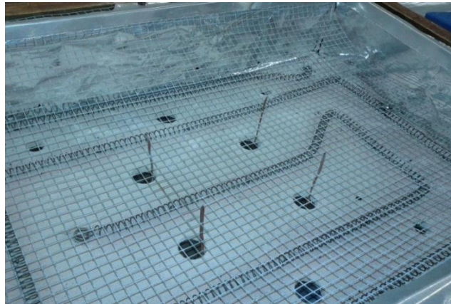
Figure 3.8: Thermocouple position on heating section.
