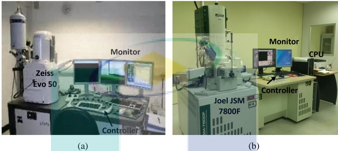
**Figure 3.6:** (a) Zeiss Evo 50 SEM. (b) Joel JSM 7800F FESEM.
