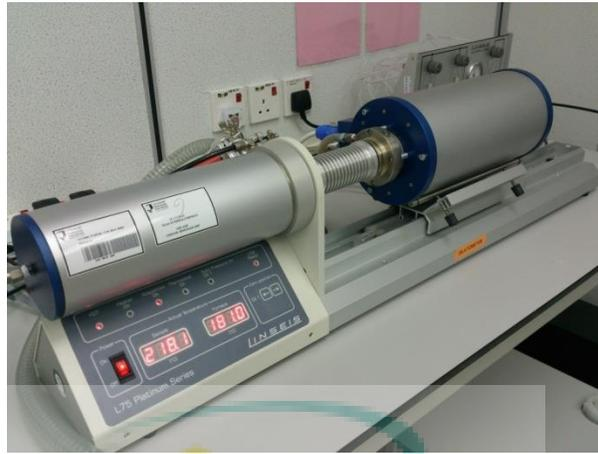
**Figure 3.8:** Linseis P75 Platinum Series dilatometer.
