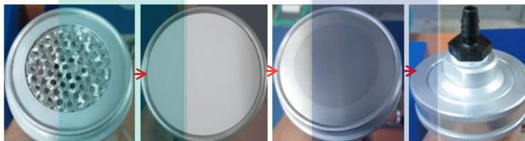
**Figure 3.10:** Placement of filter paper in filter holder
